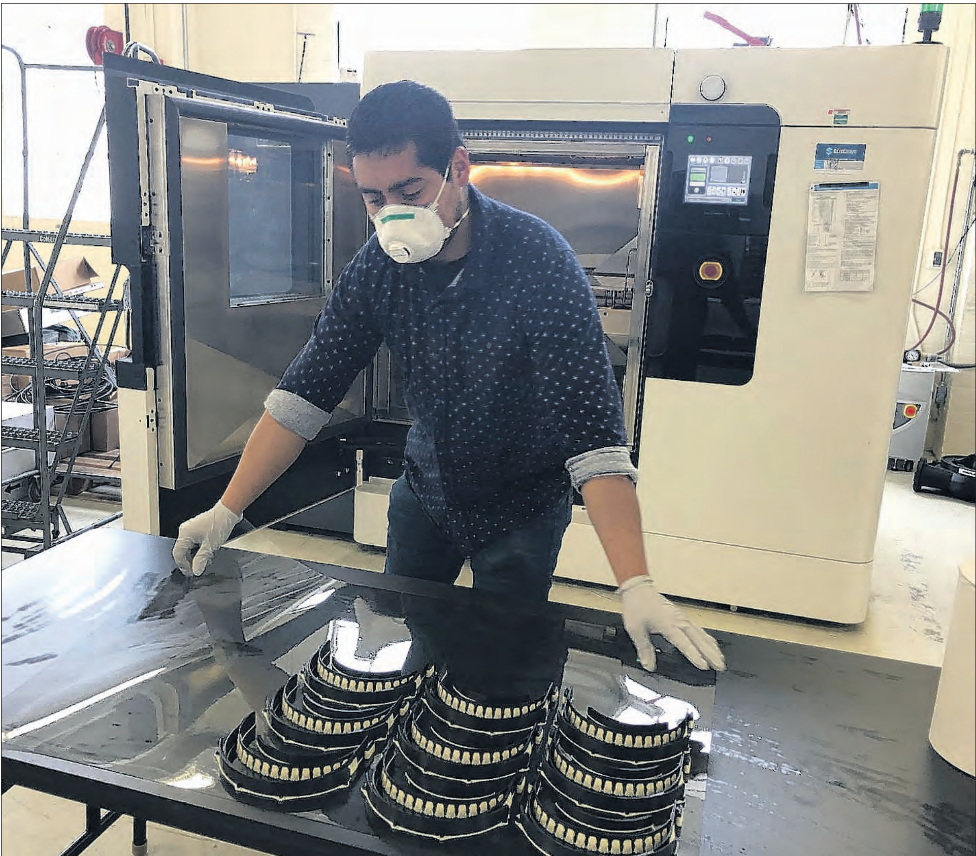
Jose Ruiz, a mechanical engineer at Naval Undersea Warfare Center (NUWC) Division Keyport, works on parts for face shield prototypes. NUWC Keyport is currently exploring ways to use its additive manufacturing capabilities to help the Washington state medical community, including Naval Hospital Bremerton, with personal protective equipment during the coronavirus pandemic. U.S. Navy photo/
