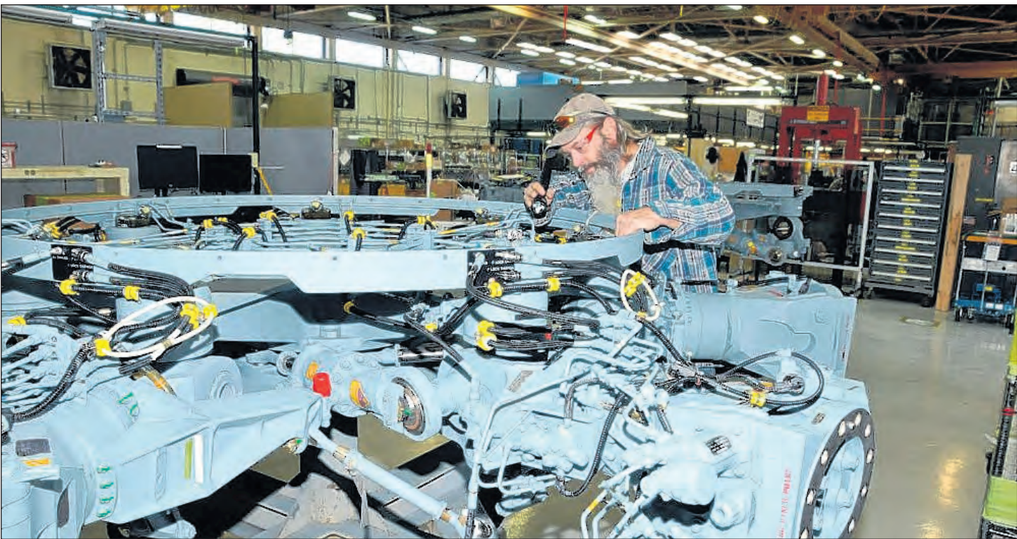
Joseph Farr, an aircraft mechanical parts repairer at Fleet Readiness Center East, inspects a completed H-53 main rotor head. FRCE recently revived its H-53 main rotor head program through a partnership with Sikorsky.
