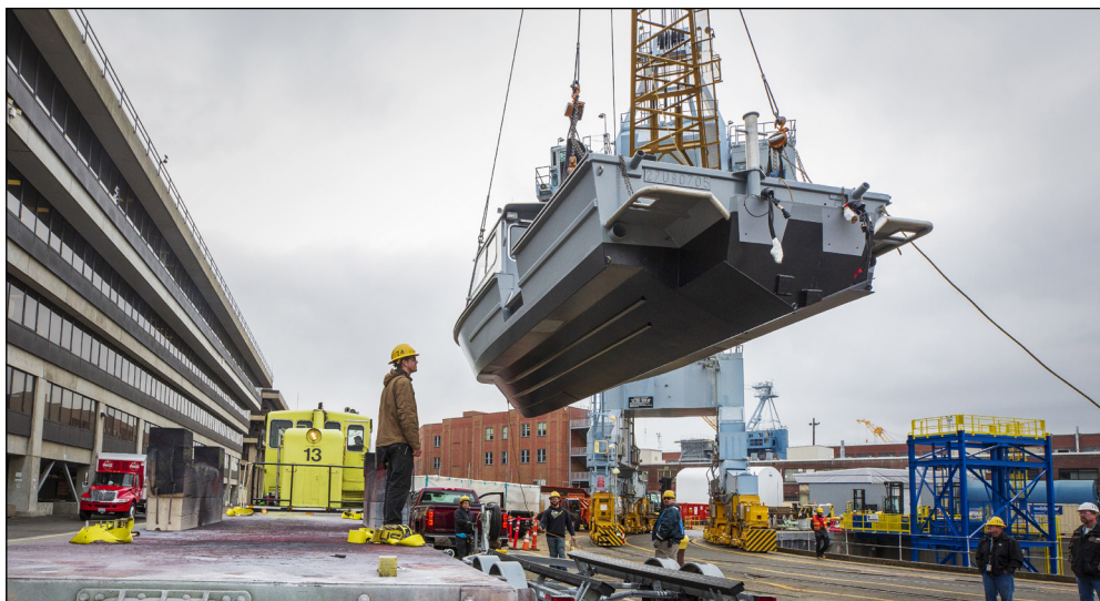
Crane Riggers from Code 740, Riggers and Operators, lift a newly modernized Dive Boat from a rail cart during a dive boat lift maneuver. The PSNS & IMF dive boat fleet was painted and modernized at the shipyard for the first time. (PSNS & IMF photos by Wendy Hallmark)
