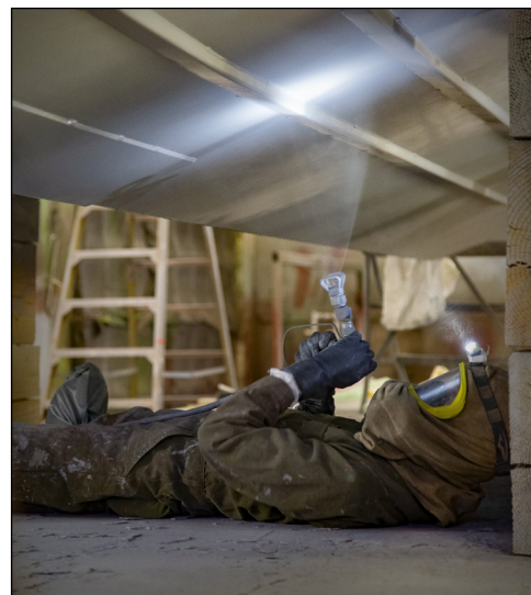
Painter Apprentice Taylor Sorensen, Shop 71, Painters, Blasters and Tile Setters, uses a spray gun to apply high-durability, long life cycle paint to a diver utility boat recently modernized at Puget Sound Naval Shipyard & Intermediate Maintenance Facility. (PSNS & IMF photos by Wendy Hallmark)
