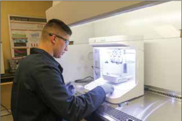
Class of 2022 Cadet Nicolas Shriver sets up a 3D bioprinter before using hydrogels to print an aortic valve. (Photo by Brandon OConnor)
