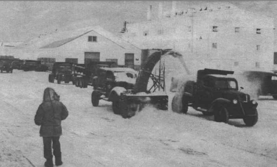
The TU3 SnoGo was produced by the Klauer Manufacturing Company of Dubuque, Iowa. It and the LTR, a mounted blade-type snow plow, were used throughout the Alaskan theater during World War II and beyond. The TU3 was an auger-style plow that could be mounted to whatever heavy duty truck was handy. It was boasted by Klauer that the TU3 could throw snow 100 feet, but the installations generally used a dump truck to collect the snow and remove it from the site entirely. Here snow is removed from Front Street in front of Hangar 1. (Photo reprinted from the Ladd Field Midnight Sun pictorial, 1945)
