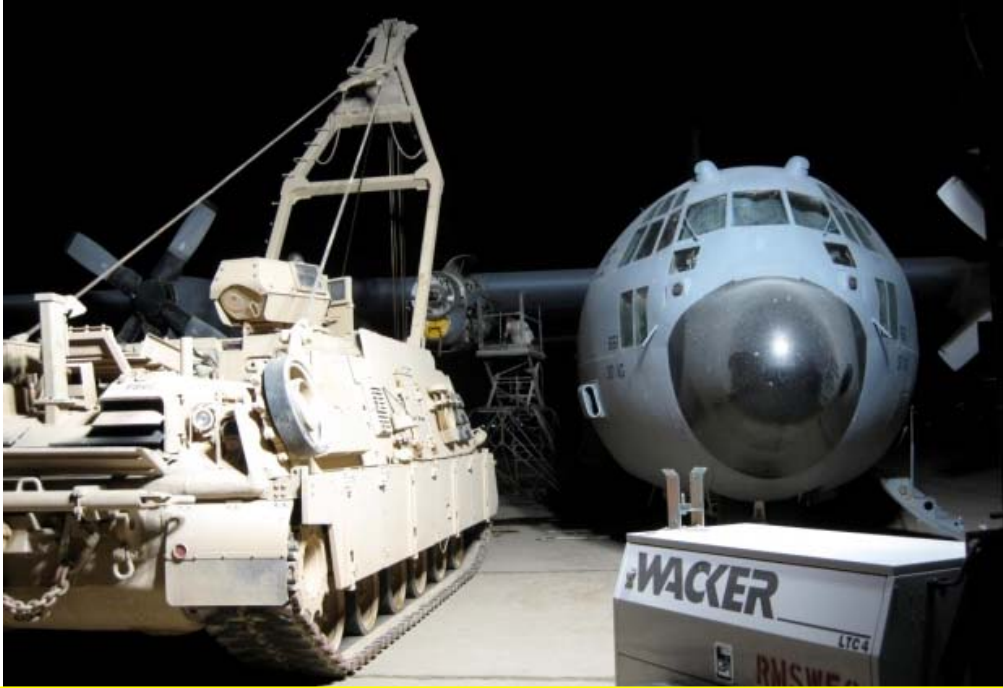
A group of Soldiers and Airmen worked night and day June 28 on Forward Operating Base Warrior, Kirkuk, Iraq, to remove the engine from a C-130. Working together the team used an Army M88A2 Hercules to pick up the engine so it could be repaired on the ground, finishing what is normally a four day job in less than 24 hours. (Photo by 2nd Brigade Combat Team, 1st Cavalry Division Public Affairs)
