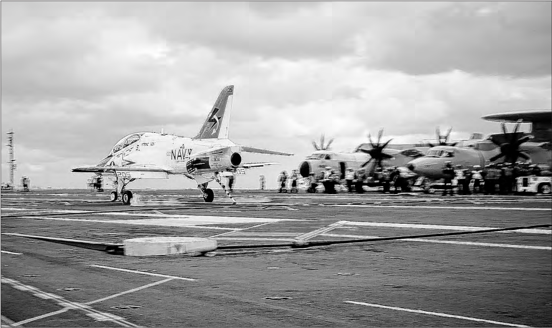
A T-45 Goshawk, assigned to Air Test and Evaluation Squadron (VX) 23, lands on USS Gerald R. Ford's (CVN 78) flight deck. Ford is currently conducting Aircraft Compatibility Testing to further test its Electromagnetic Aircraft Launch Systems (EMALS) and Advanced Arresting Gear (AAG). MC3 Ryan Carter
