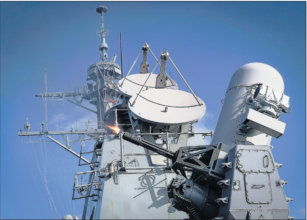
MCSN Darcy McAtee The Arleigh Burke-class guided-missile destroyer USS Mason (DDG 87) fires live rounds from its Mark 15 Phalanx close-in weapons system (CIWS). Mason is underway with Norfolk-based cruiser-destroyer (CRUDES) units from Carrier Strike Group 12 conducting a Live Fire With a Purpose (LFWAP) event.
