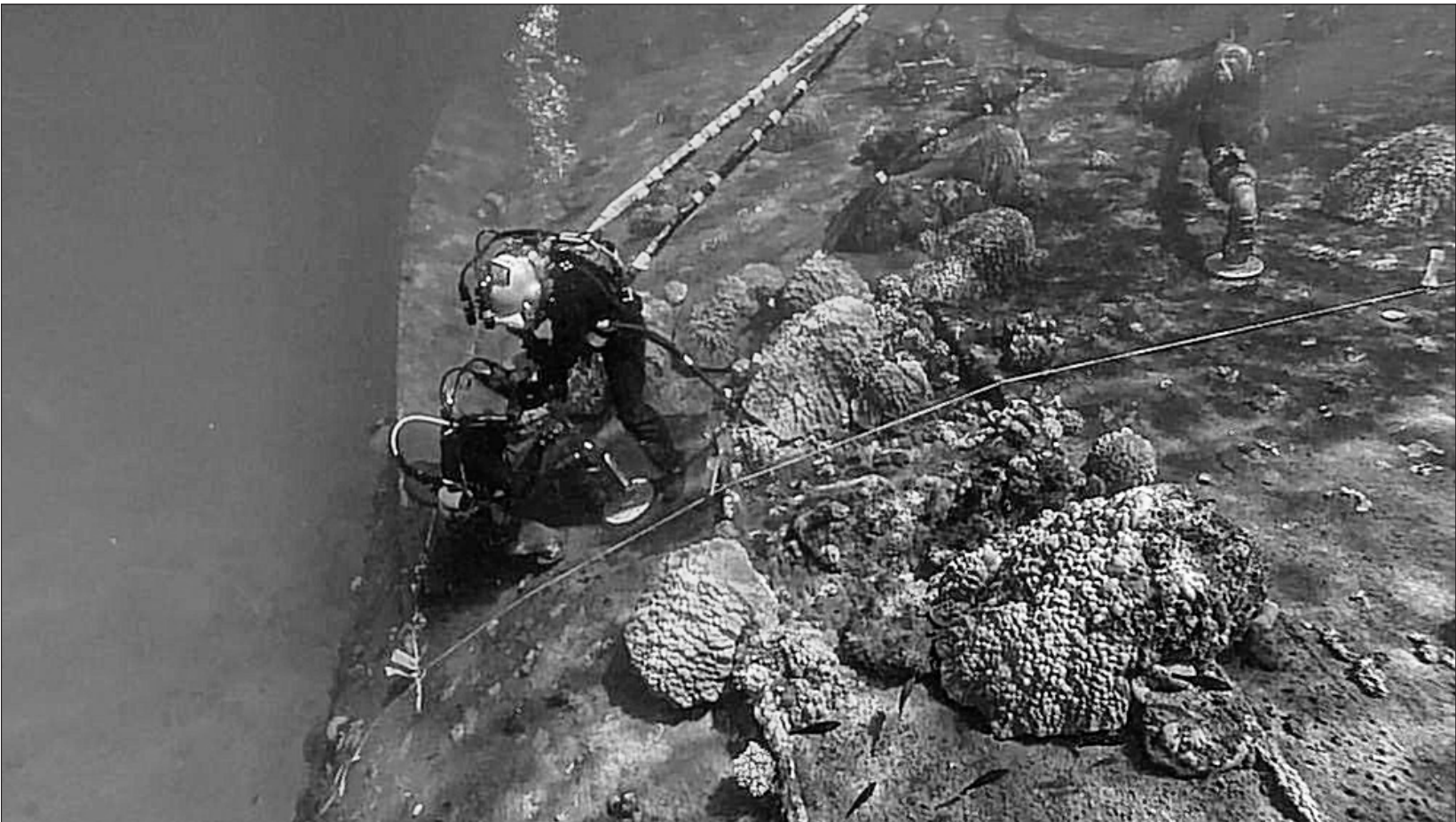
Navy divers from Mobile Diving Salvage Unit (MDSU) 1, aboard USNS Salvor (T-ARS-52), remove fuel oil from the capsized World War II German cruiser Prinz Eugen. The safe extraction of an estimated 250,000 gallons of fuel oil from Prinz Eugen began Sept. 1 and involved nearly two dozen divers along with support from commercial tanker Humber in collaboration with the government of the Republic of the Marshall Islands and U.S. Army Garrison Kwajalein Atoll.
