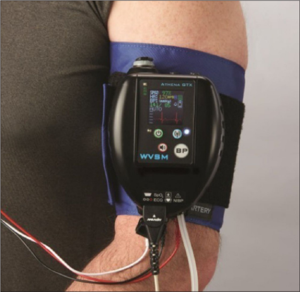
Courtesy Athena GTX The Wireless Vital Signs Monitor (WVSM). Sponsored by the Office of Naval Research, the WVSM tracks critical health information like heart rate, pulse and blood pressure. It weighs less than a pound and can be carried easily into combat zones or mass-casualty emergency situations.
