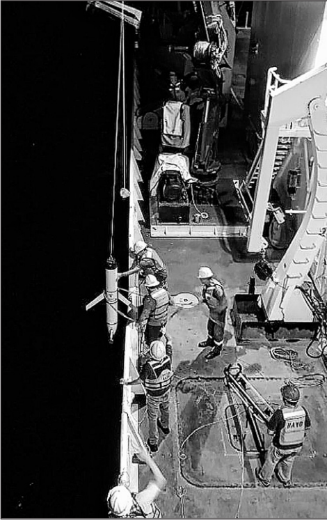
U.S. Navy photo USNS Bowditch crew members and Naval Oceanographic Office surveyors conduct routine night operations recovering a littoral battlespace sensing glider in the Philippine Sea. These gliders can collect environmental data, such as water temperature and salinity, for months at a time without the need for active propulsion.
