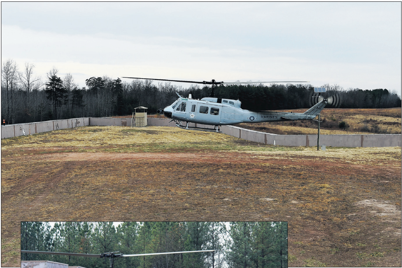
Marines offload cargo from a UH-1 Huey equipped with an Office of Naval Research-sponsored Autonomous Aerial Cargo/Utility System (AACUS) autonomy kit following a landing during final testing at Marine Corps Base Quantico.
