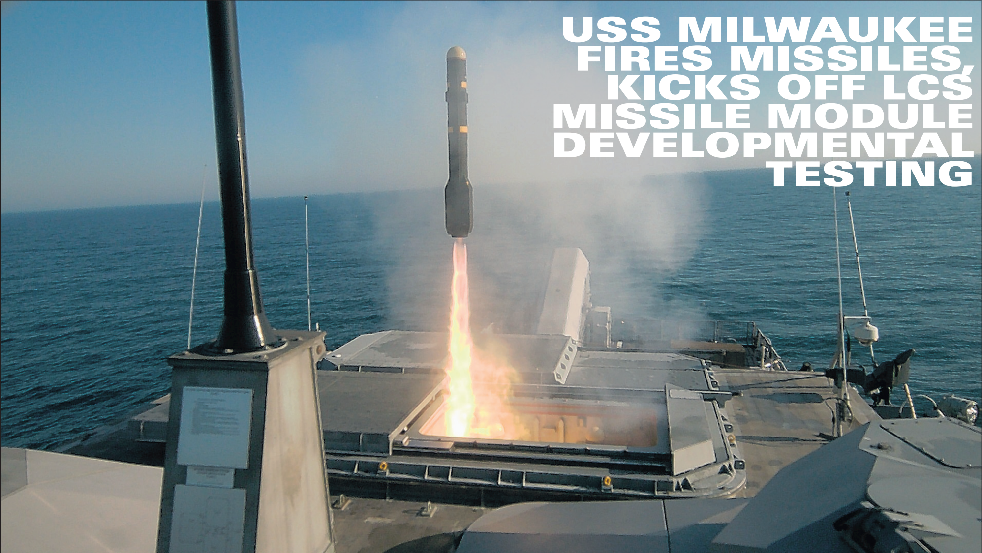
U.S. Navy photo The Freedom-variant littoral combat ship USS Milwaukee (LCS 5) fires an AGM-114L Longbow Hellfire missile during a live-fire missile exercise off the coast of Virginia, May 11, 2018. Milwaukee fired four Longbow Hellfire missiles that successfully struck fast inshore attack craft targets during a complex warfighting environment utilizing radar and other systems to track the targets.
