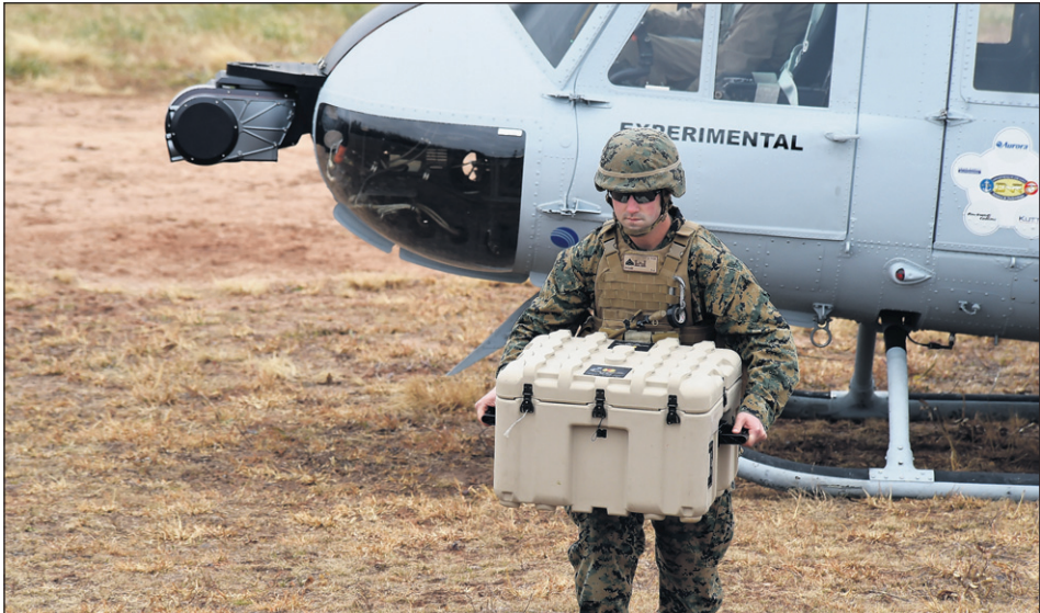
A Marine offloads cargo from a UH-1 Huey equipped with an Office of Naval Research-sponsored Autonomous Aerial Cargo/Utility System (AACUS) autonomy kit following a landing during final testing at Marine Corps Base Quantico.
