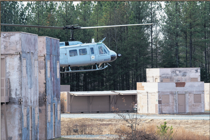
A UH-1 Huey equipped with an Office of Naval Research-funded Autonomous Aerial Cargo/Utility System (AACUS) autonomy kit lands within the walls of a Forward Operating Base during final testing at Marine Corps Base Quantico.
