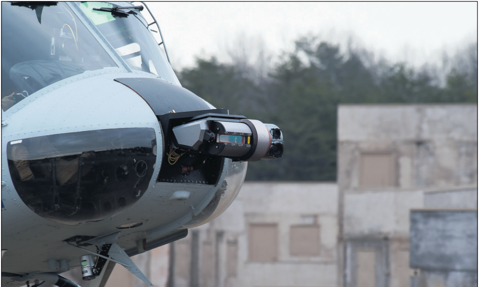
A UH-1 Huey equipped with an Office of Naval Research-sponsored Autonomous Aerial Cargo/Utility System (AACUS) autonomy kit makes an approach for landing during final testing at Marine Corps Base Quantico.
