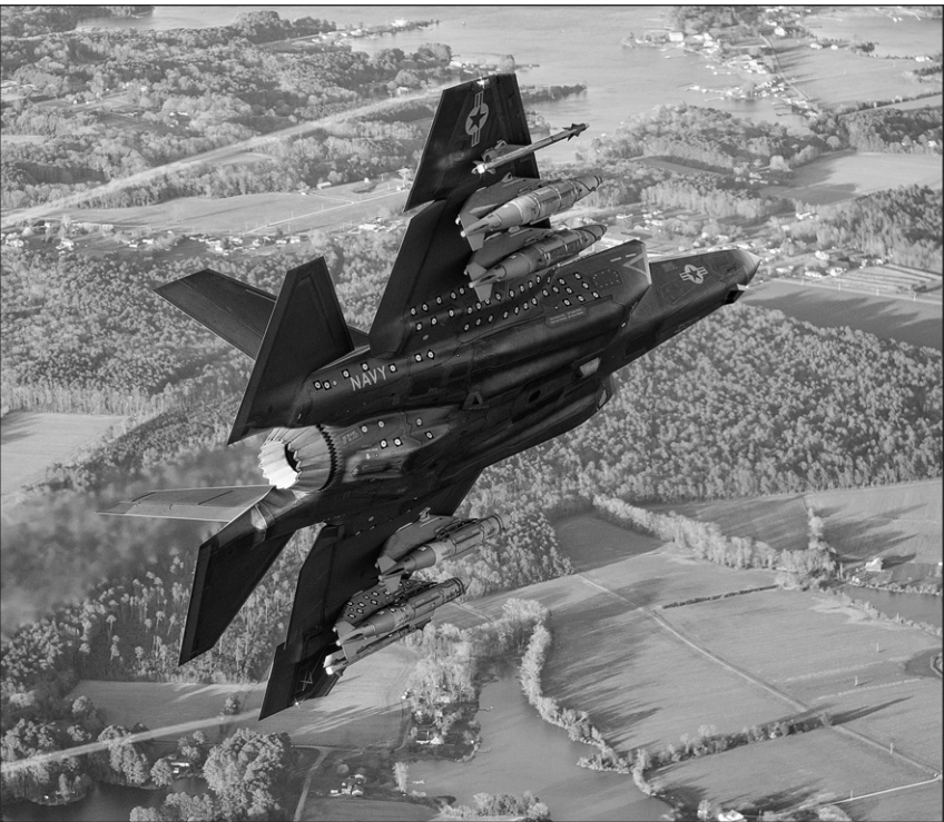
Test pilot Billie Flynn pilots an F-35C Lightning II test aircraft during an external GBU-31 and AIM-9x buffet and flutter test flight from Naval Air Station Patuxent River, Md. Dane Wiedmann
