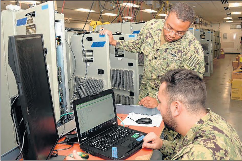
Rick Naystatt U.S. Navy Information Systems Technicians 2nd Class Jchaun Rountree, left, and Hakan Ozdemir, perform operational checks on Consolidated Afloat Ships Network Enterprise Services (CANES) racks bound for their ship, the aircraft carrier USS Ronald Reagan (CVN 76) in Naval Information Warfare Center Pacific's Network Integration and Engineering Facility.
