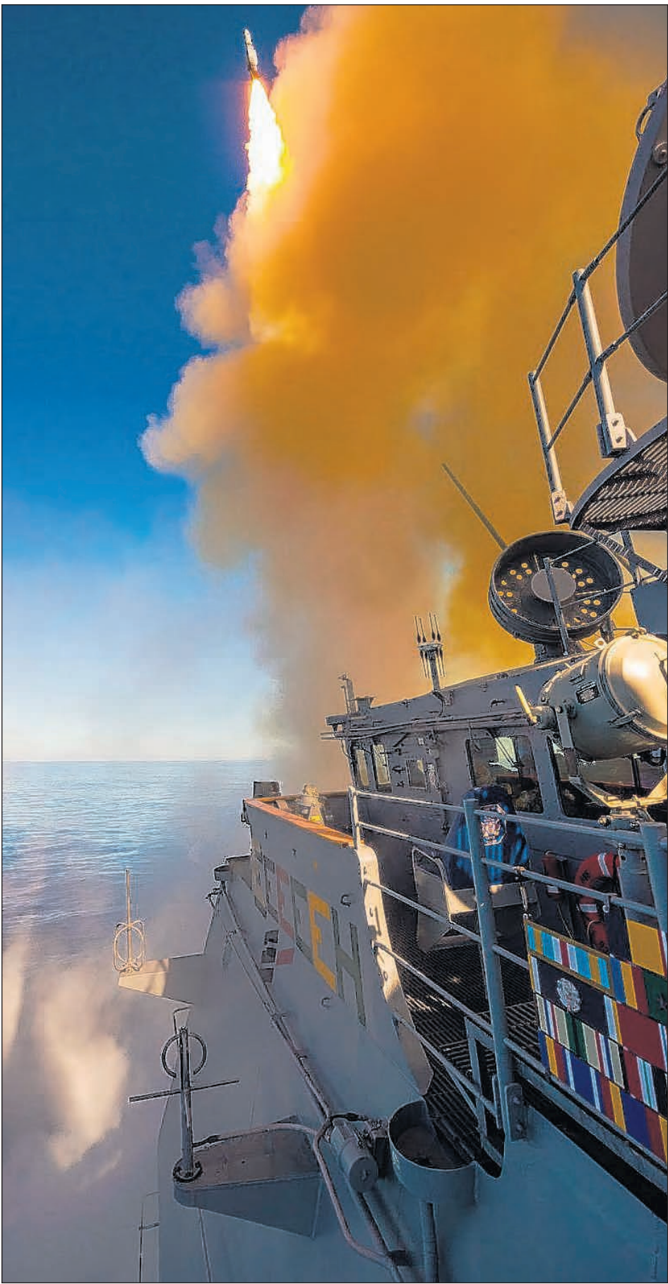
MC1 Chad M. Butler An SM-2 missile launches and destroys an airborne training target during a successful first test of the updated AEGIS Baseline 9 weapons system aboard the guided-missile cruiser USS Mobile Bay (CG 53). Mobile Bay, the first guided-missile cruiser in the fleet to upgrade from AEGIS Baseline 8 to the updated Baseline 9, is underway testing new weapons capabilities in preparation for its upcoming deployment.
