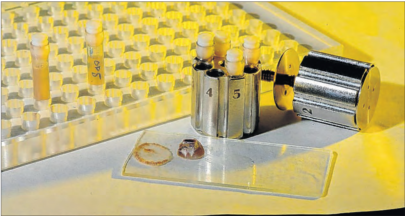
Barnacle samples in pressure cycling technology (PCT) tubes and bullet with barnacle samples in the background are used for proteomics analysis at U.S. Naval Research Laboratory, Washington, D.C. August 2. The barnacle base plate covers the glue, illustrating how difficult sample collection is; the tubes and bullet are specially designed to handle high pressure conditions.
