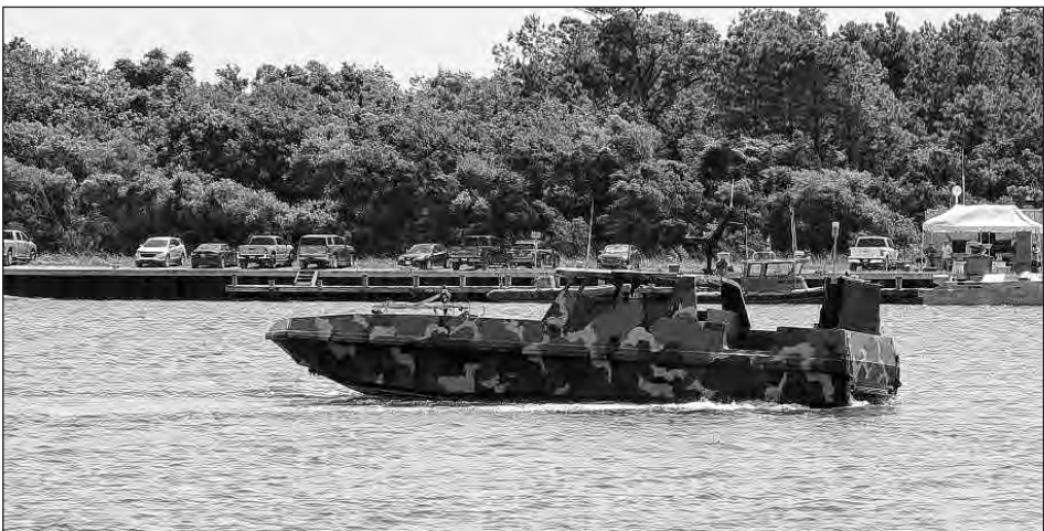
Kelley Stirling Combatant Craft Division, a detachment of Naval Surface Warfare Center, Carderock Division, demonstrates the Unmanned Surface Vehicle Lab Afloat on July 17, during the Advanced Naval Technology Exercise (ANTX) East in Camp Lejeune, N.C. The USV Lab Afloat is a key component to the USV Autonomy Lab and Integration Center, and while at ANTX East, the boat docked itself autonomously.
