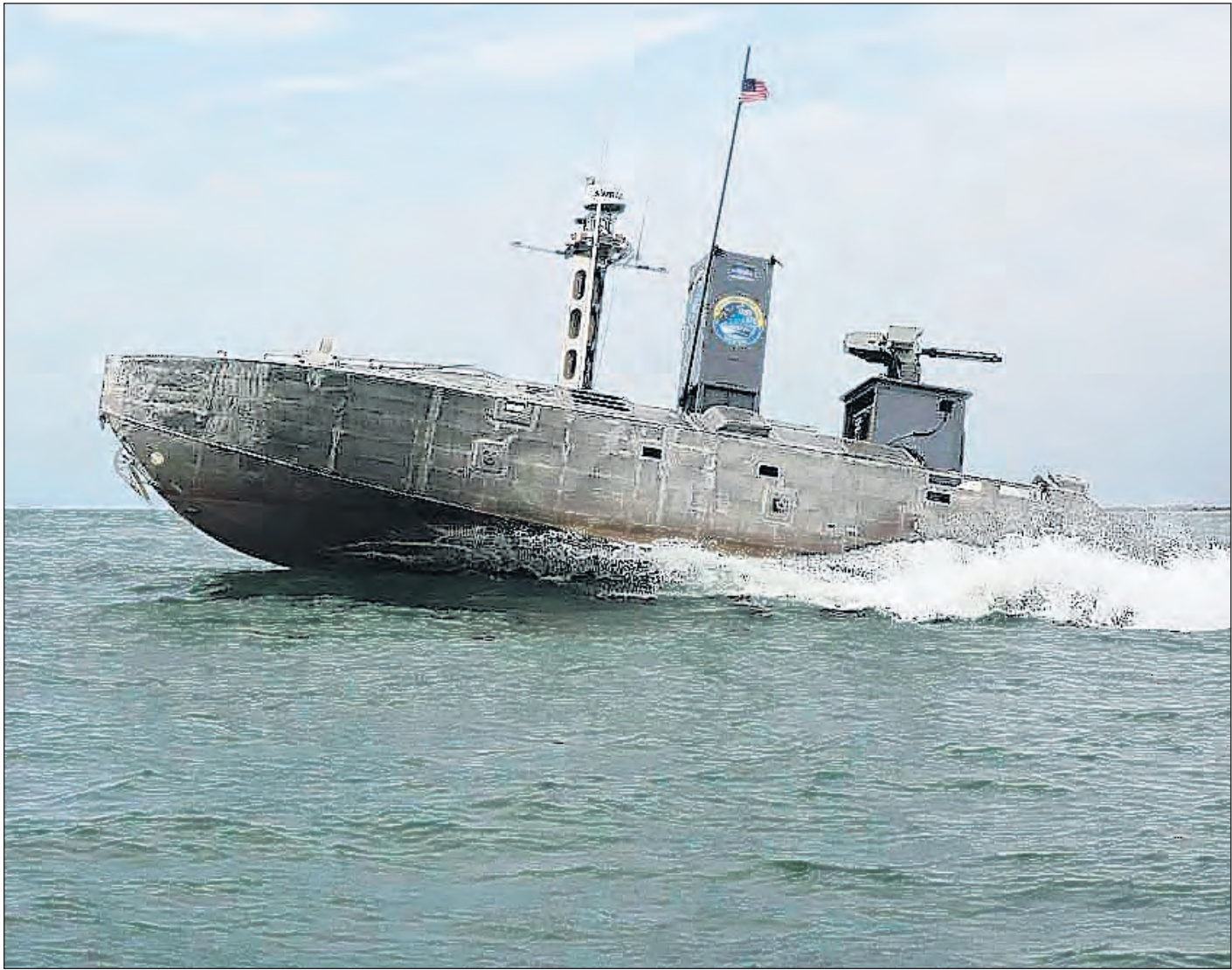
LCpl. Nicholas Guevara An Expeditionary Warfare Unmanned Surface Vessel (USV) autonomously navigates a predetermined course through the water during Advanced Naval Technology Exercise 2019 at Camp Lejeune, N.C. July 12. ANTIX East 2019 is an event designed to test new technology with academic, industry and Navy participants.
