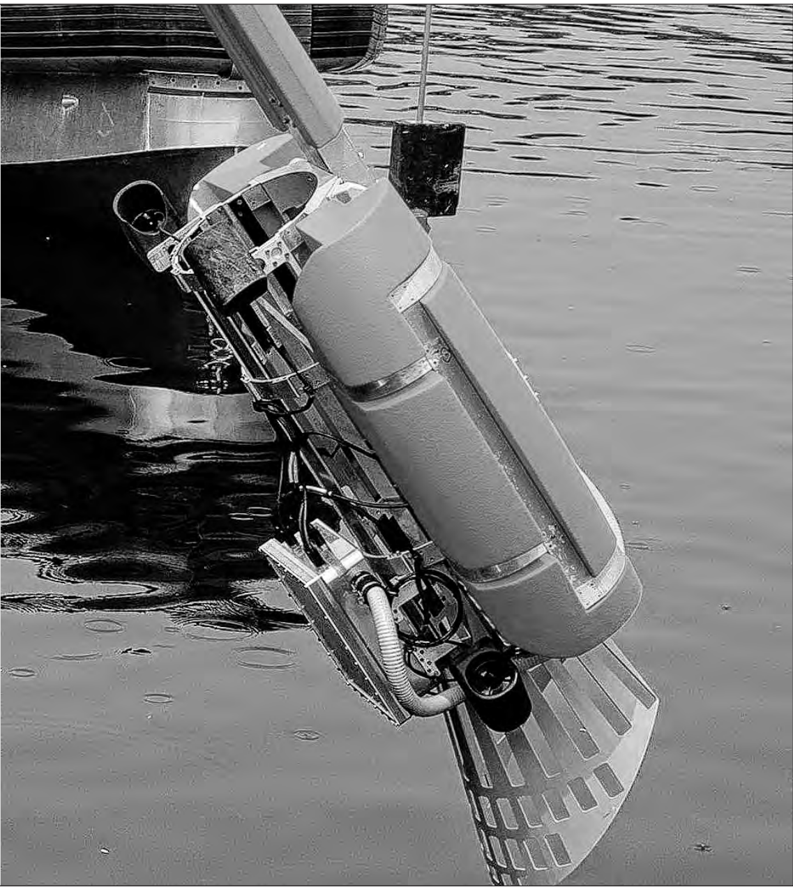
Ashley Conner The Airborne Surface Quad Thruster Interface Device, or ASQUID, attaches to the side of a MH-60 helicopter and allows the crew to lowers a MK-18 into the water to search for mines preventing Navy personnel from having to enter a minefield.
