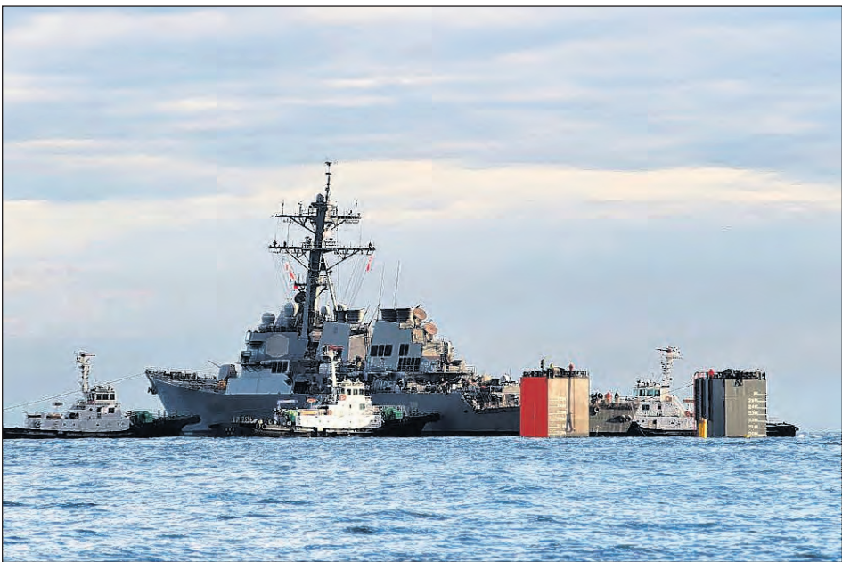
MC2 William McCann The Arleigh Burke-class guided-missile destroyer USS Fitzgerald (DDG 62) is loaded onto the heavy lift transport MV Transshelf. Transshelf will transport Fitzgerald to Pascagoula, Mississippi to complete repairs.
