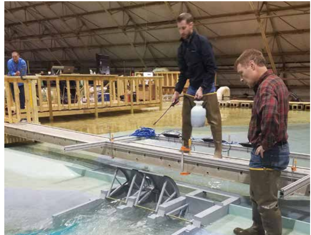
Kevin Denn, engineering and construction, left, and Aaron Buesing, engineering and construction, run tests on the Fargo-Moorhead Flood Risk Management Project Red River Structure model at the Engineering Research and Development Center and their Coastal and Hydraulics Laboratory in Vicksburg, Mississippi. Courtesy photo
