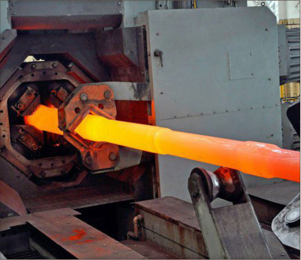
After being heated to nearly 2000 degrees, an M1 Abrams tank 120mm cannon tube is formed with Watervliet Arsenal, New York's, rotary forge.
