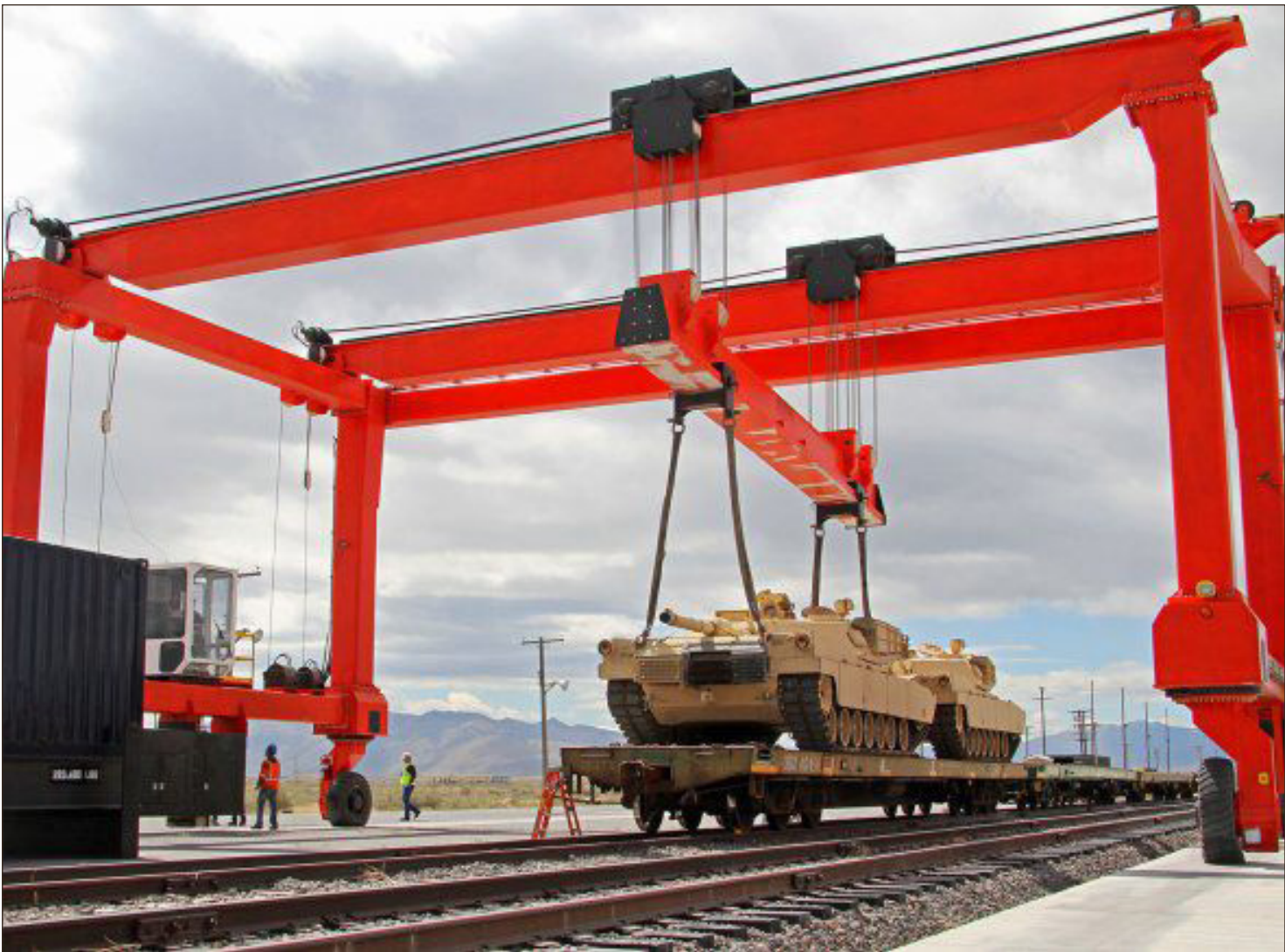
M1 Abrams tanks are loaded onto rail cars using the high capacity gantry crane at Sierra Army Depot, California.
