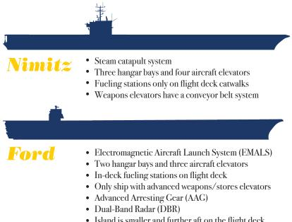
Island is smaller and further aft on the flight deck
