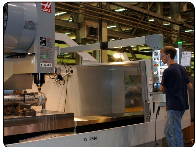
A Watervliet machinist performs a vertical milling operation on a cannon. (U.S. Army photo by William Martin)
