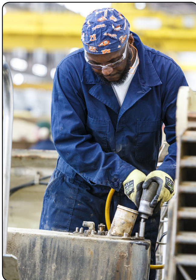
Tyrone Garrett removes the rear sending unit from a rear fuel cell on a M1A2 in Anniston Army Depot's Combat Vehicle Repair Facility. (U.S. Army photo by Mark Cleghorn)
