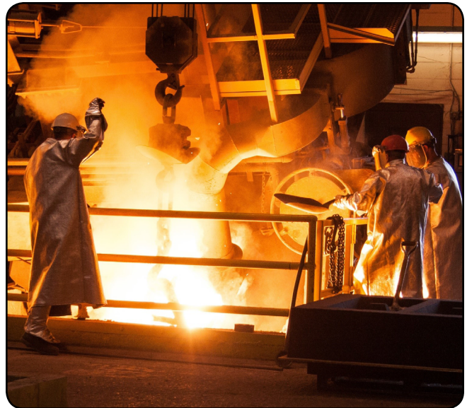
Rock Island Arsenal-Joint Manufacturing and Technology Center foundry employees conducted a test pour to prove out a new pour basin for the M777 howitzer muzzle break at Rock Island Arsenal, Illinois. The new muzzle break casting is designed by the University of Iowa. In addition to the muzzle break, pours for test plates used to certify weld processes on the muzzle break and test bars used to verify heat-treat processes were completed. This effort is working to improve muzzle break pours, producing the finest products for the warfighter. (U.S. Army photo by Debralee Best)
