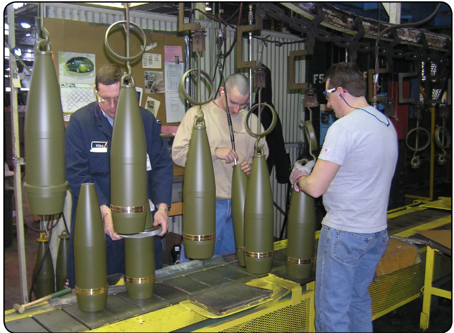
Painted ammunition parts that have dried in an oven are unloaded from the conveyor to be placed on pallets for shipping. A Quality Assurance Specialist is checking the paint thickness to ensure it meets requirements. (U.S. Army photo)
