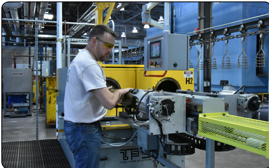
A U.S. Navy Indian Head employee loads obsolete MK9 cartridge cases as a part of the retrofitting process to recycle old cartridge cases into modernized MK109 versions to accommodate new propellant for the Navy. (U.S. Army photo by Dori Whipple)
