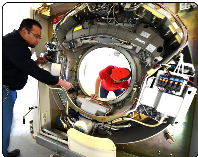
LEFT: Medical maintenance experts at Medical Maintenance Operations Division-Tracy, under the U.S. Army Medical Materiel Agency, inspect a computerized tomography system that recently arrived to the depot for recapitalization. (U.S. Army photo by Ellen Crown)
