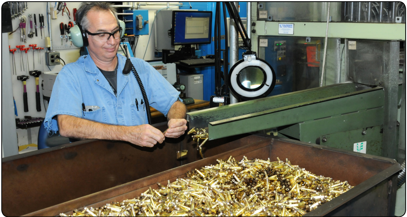
A contractor employee at Lake City Army Ammunition Plant (LCAAP), Missouri, inspects small-caliber cartridge cases during production. LCAAP provides quality small-caliber munitions to the warfighter in support of global operations. (U.S. Army photo by Tony Lopez)
