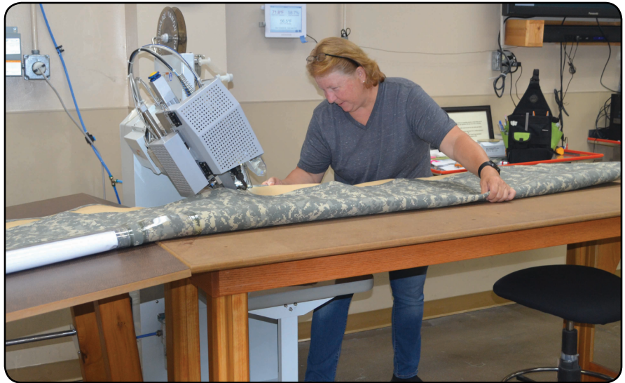
An employee with Pine Bluff Arsenal's Directorate of Chemical and Biological Defense Operations seam seals a protective patient wrap at the Arsenal's Chemical Protective Clothing Production Facility. (U.S. Army photo by Rachel Selby)
