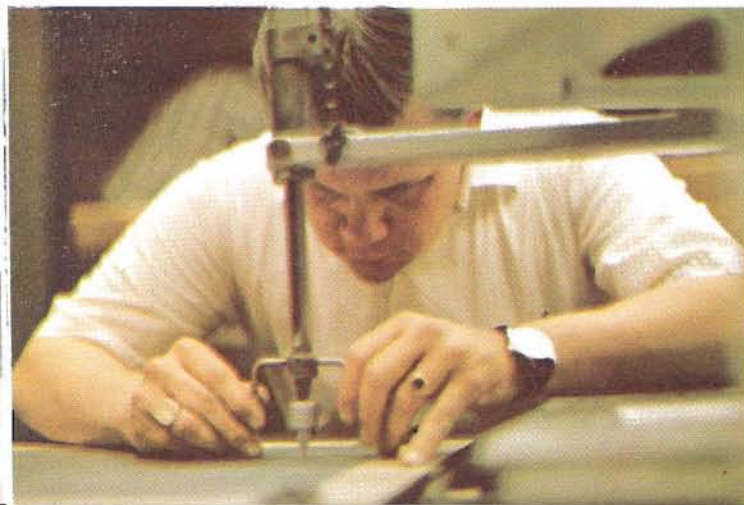
A technician tracing map relief with a "pantograph router" . . . The information received is transformed into 3 dimensional figures.
