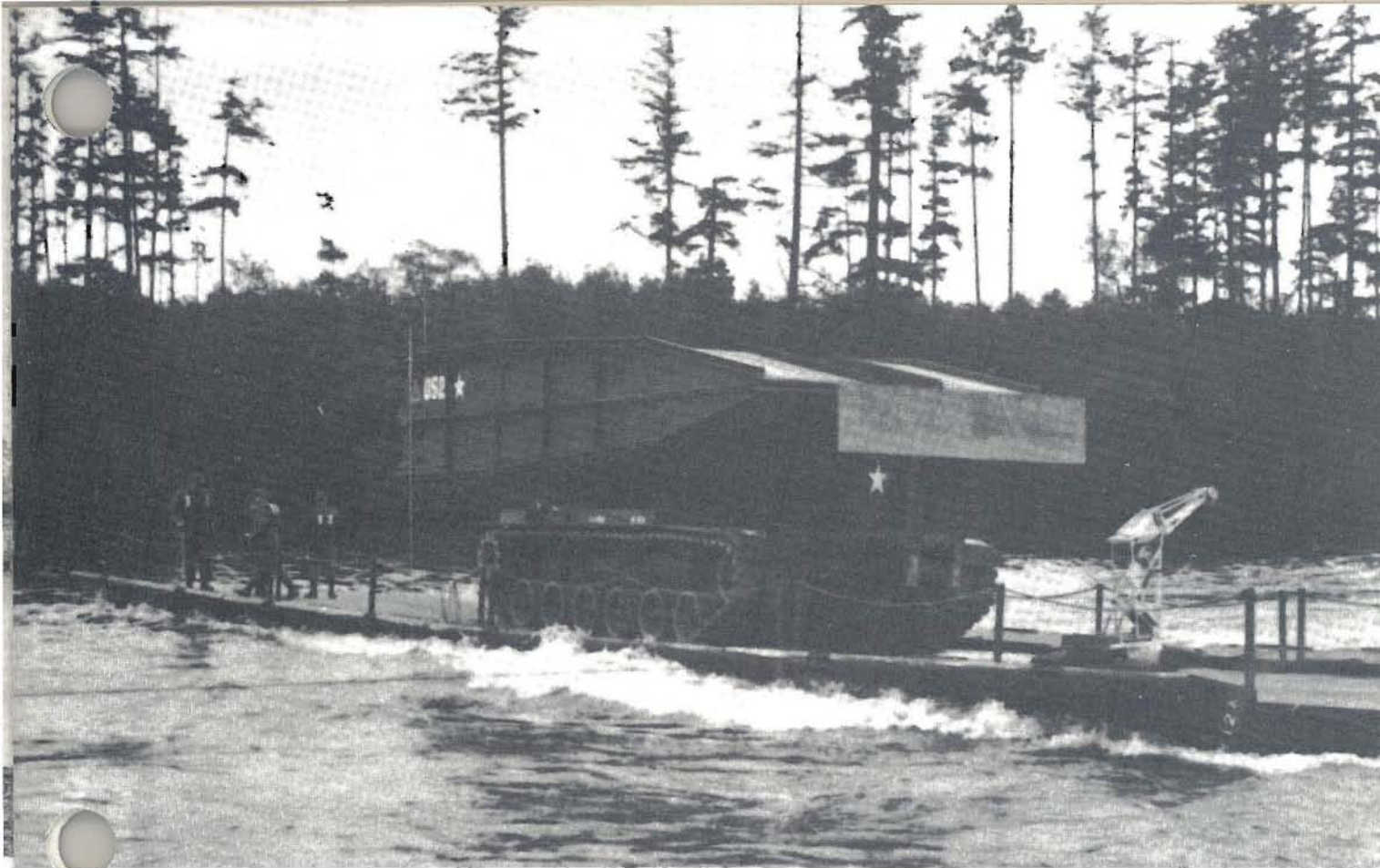
Sections of the Ribbon Bridge being used as a power raft to expedite the river crossing of an Armored Vehicle Launched Bridge (AVLB).
