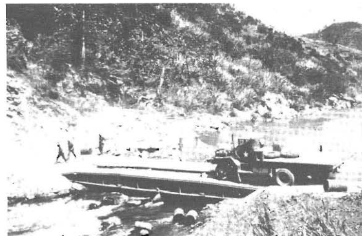
Engineers span a tributary of the Quan Tri River with an AVLB.
