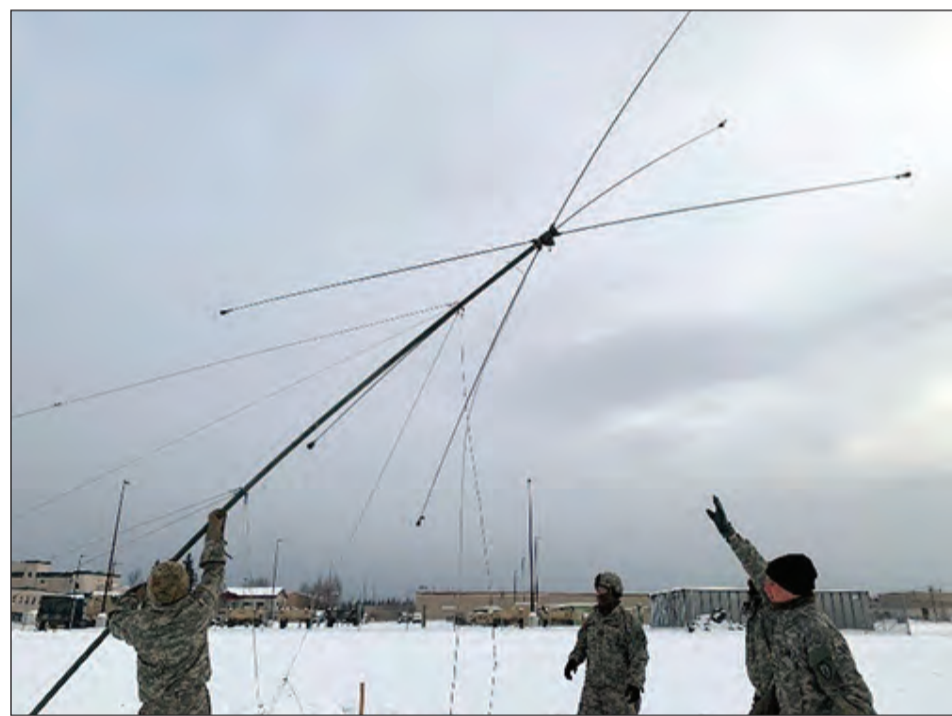
Team leader, Spc. Rutherford, Charlie "Lightning" Company 70th Brigade Engineer Battalion, explains to his team the set-up and completion process of the OE-254. Team members assume their position on the antenna as they raise it, bringing the antenna to an upright position, where it is now ready to help aid in the receiving and sending of communications. (Courtesy photo)
