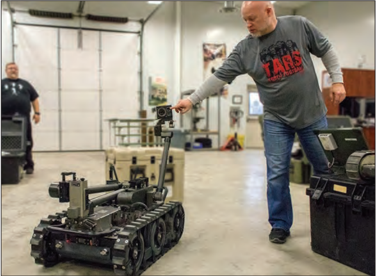
Bill Hagerty, Robotics University new equipment trainer, points to the new thermal vision camera atop the MTRS Inc II robot. The robot will soon replace its predecessor, the Talon 5 and boasts an array of improvements. (Photo by Sam Campbell)
