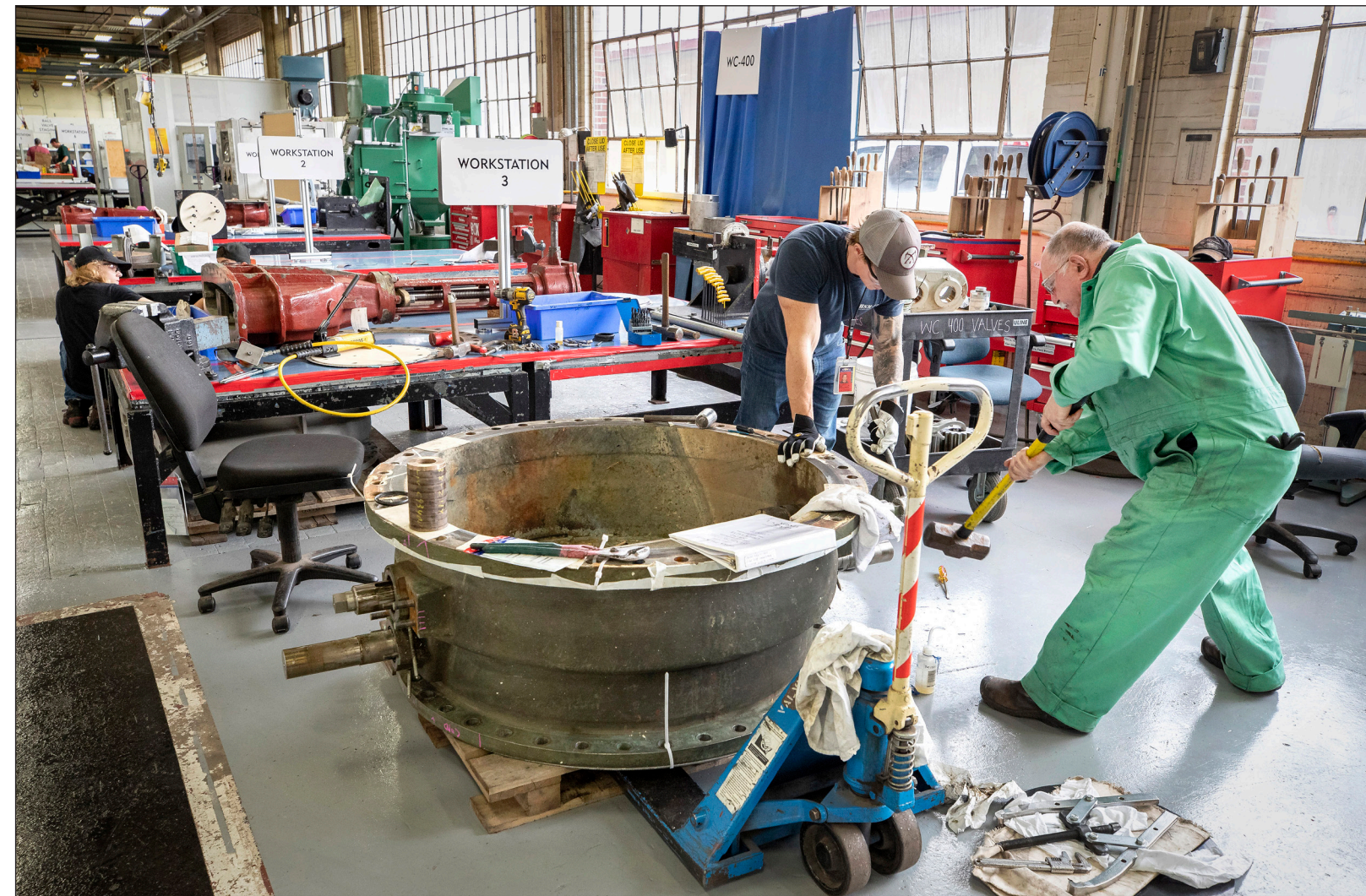
Bench Mechanic Emil Skarpona, right, Shop 31, Inside Machine Shop, works with Devan McNeilly to repair a check valve in the Work Center 400 floor space inside Building 431. (PSNS & IMF photo by Scott Hansen)
