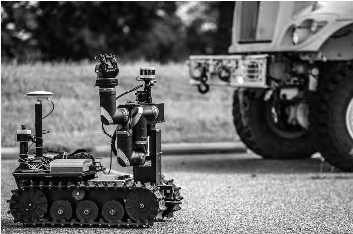
RoMan, short for Robotic Manipulator, is a tracked robot with arms and hands – necessary appendages to remove heavy objects and other road debris from military vehicles’ paths. (Photo by David McNally)
