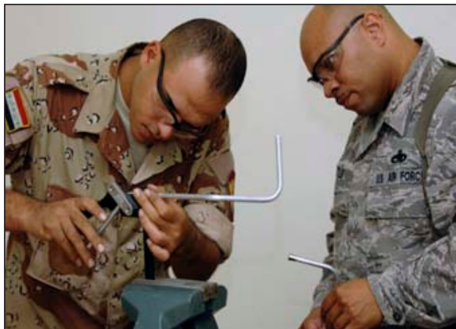
Master Sgt. Joel Little watches Iraqi air force warrant officer, Omar Saaed bend a piece of metal tubing during the fabrication portion of the aircraft structural maintenance course at Al-Taji Air Base, Iraq, Jan. 5. Little is deployed with the 821st Air Expeditionary Training Squadron. (U.S. Air Force photo by Staff Sgt. Paul Villanueva II)
