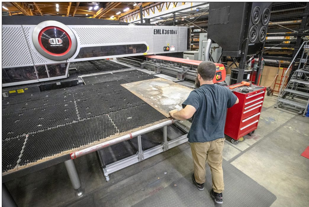
Chris Bamonte, Shop 17, Sheet Metal Shop, mechanic prepares to cut a piece of sheet metal using the automated laser cutter inside Building 857. (PSNS & IMF photo by Scott Hansen)
