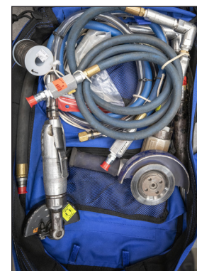
A typical job kit includes grinders, a needle gun, wrenches hangers and glass tape.
