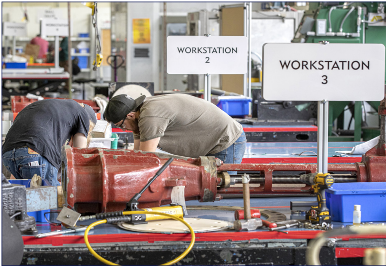
Improvements to work center 400, in Shop 31, Inside Machine Shop, located in Bldg. 431, provides a more open floor plan allowing better visibility of the work. The changes also brought the test flanges closer to the test benches improving employee safety. (PSNS & IMF photo by Scott Hansen)
