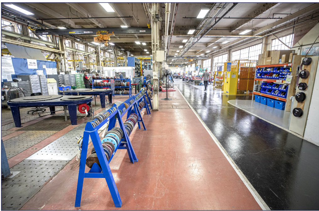
Improvements to work center 400, in Shop 31, Inside Machine Shop, located in Bldg. 431, provides a more open floor plan allowing better visibility of the work. The changes also brought the test flanges closer to the test benches improving employee safety. (PSNS & IMF photo by Scott Hansen)
