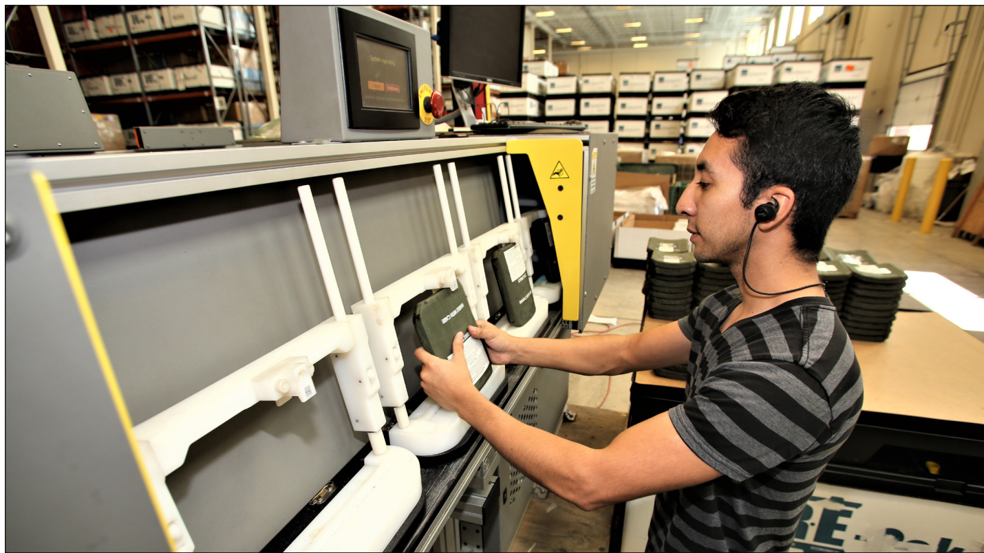
Chris Alvarado with Army contractor IAP Services places a piece of body armor into an Armor Inspection System X-ray machine Sept. 16 at the Central Issue Facility at Fort McCoy.
