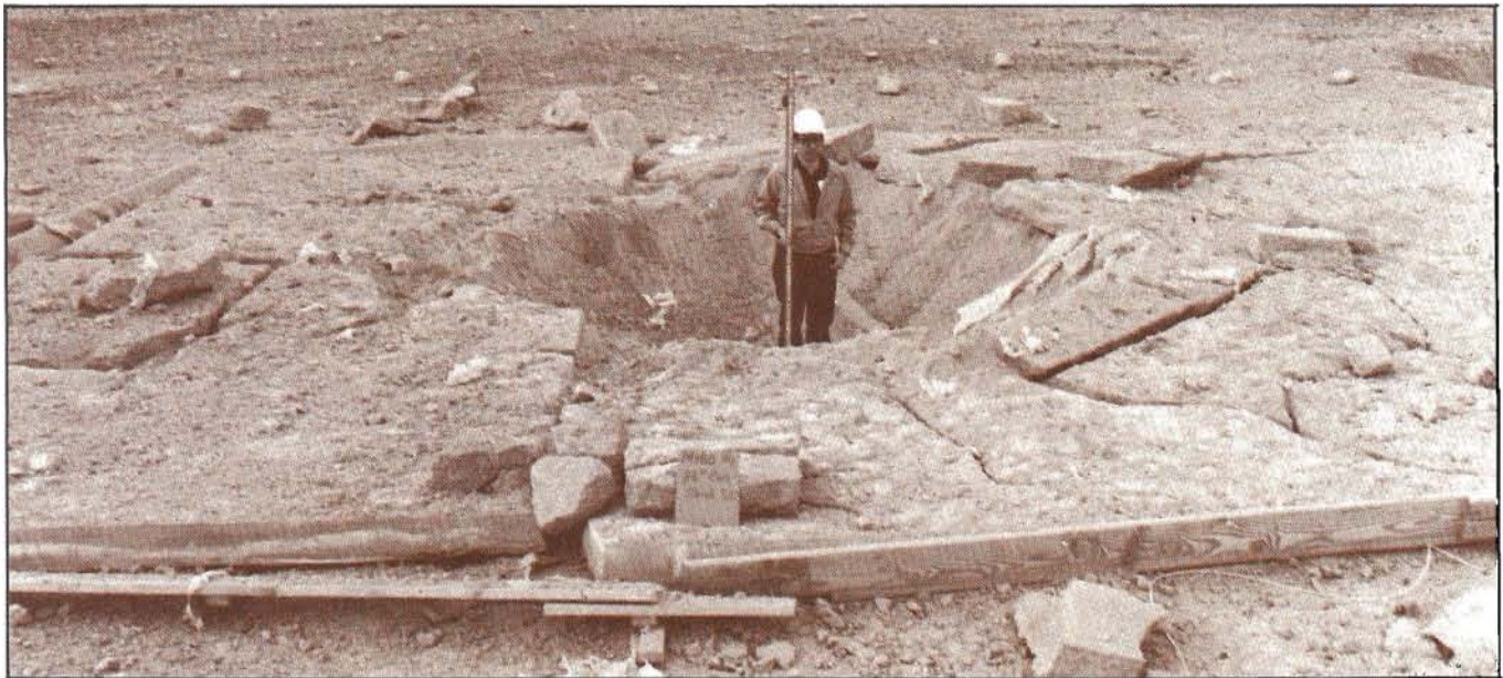
FIGURE 6 Single M180 crater in 7.5-inch concrete pavement
