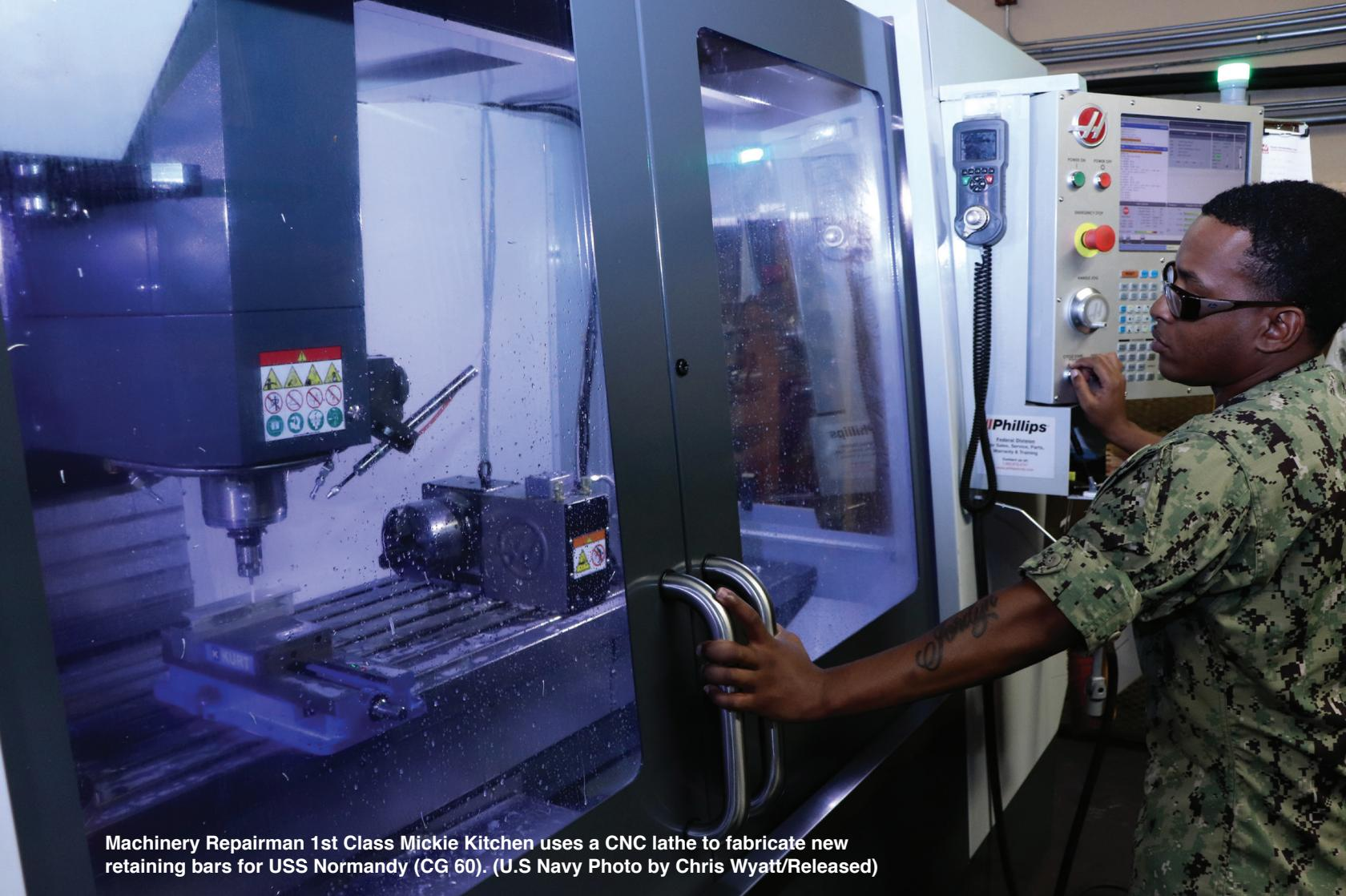
Machinery Repairman 1st Class Mickie Kitchen uses a CNC lathe to fabricate new retaining bars for USS Normandy (CG 60). (U.S Navy Photo by Chris Wyatt/Released)
