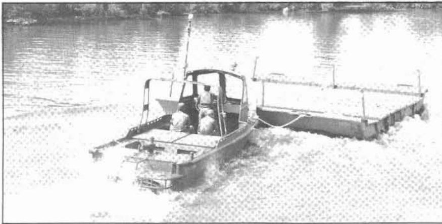
Engineers can build the ribbon bridge in shallow water because of the new boat's 22-inch draft (U.S. Army photo).
