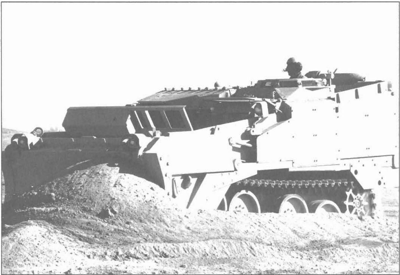
When operated according to standard, the M9 ACE is a safe and effective piece of equipment. Here, an operator is not using the M9 ACE according to standard; he did not fill the bowl with dirt for ballast.
