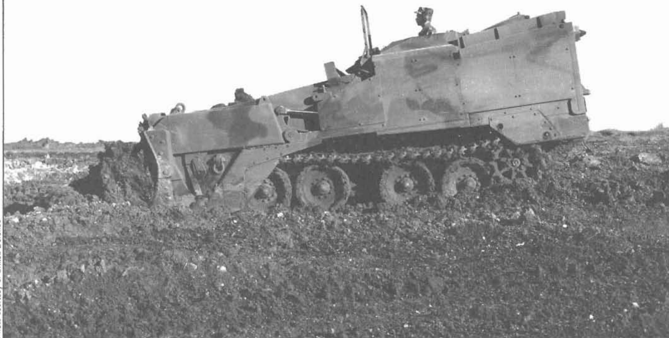
The M9 ACE is used to dig a vehicular fighting position.
