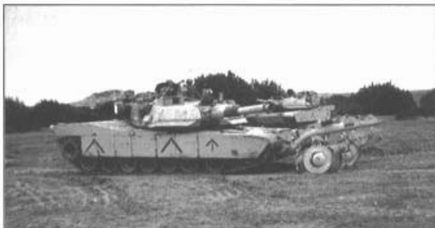
An A/3-67 Armor M1A1 moving to a company assembly area. Note the deliberate orientation of the gun tube away from the roller assembly.
