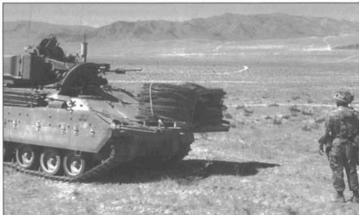
A Bradley vehicle transporting bundles of wire on its trim vane.
