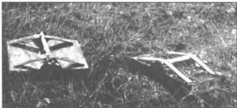
A German World War I vintage antitank mine lifted by U.S. combat engineers prior to its destruction. (Photo courtesy of Military Engineer magazine)
