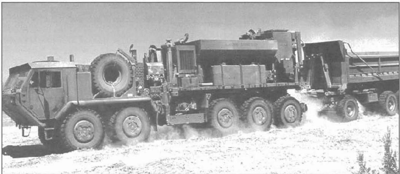
The versatility of the PLS system with EMMs is depicted in this photo of the EMM concrete mobile mixer with PLS dump body. Upon arrival at the work site, the PLS truck can off-load the concrete EMM for stationary operation, then load the dump body from the trailer to perform dump operations.
