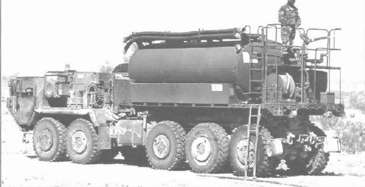
The EMM water-distributor module is intermodal transportable and is powered by its own diesel engine. It has a 3,000-gallon, stainless-steel tank and is equipped with a self-loading, 600-gallons-per-minute pump unit. The water cannon's 175-foot spray range complements the 50-foot hose and nozzle.
