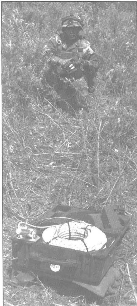
The lightweight mobile obstacle breacher will clear a path 250 feet long and 18 inches wide.
