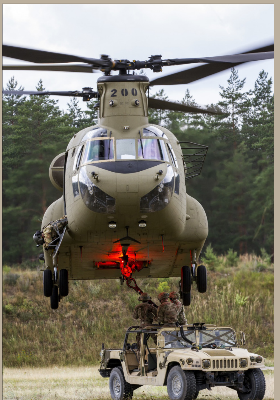
Sgt. Jeremiah Woods | 358TH PAD Soldiers with Company E, 1st Engineer Battalion, 1st Armored Brigade Combat Team, 1st Infantry Division, hook a Humvee to a CH-47 Chinook belonging to 2nd General Support Aviation Battalion, 1st Aviation Regiment, 1st Combat Aviation Brigade, 1st Inf. Div., during a sling load training exercise on a range at Grafenwoehr Training Area, Germany, July 30. Training to sling load vehicles and equipment in the field is an essential part of the combat readiness mission of the 1st Eng. Bn., 1st ABCT, 1st Inf. Div., during Atlantic Resolve.
