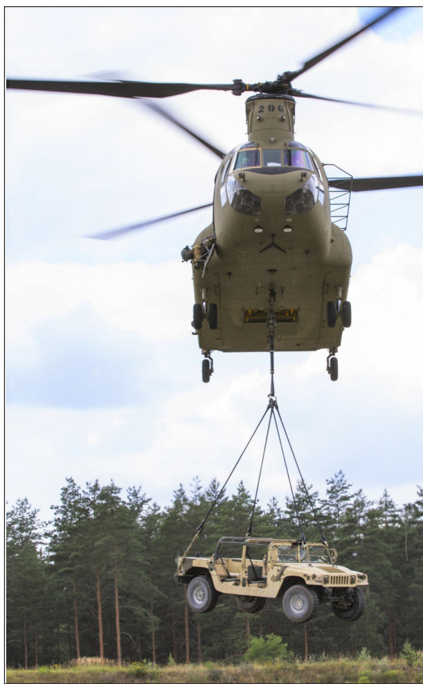
A CH-47 Chinook belonging to 2nd General Support Aviation Battalion, 1st Aviation Regiment, 1st Combat Aviation Brigade, lifts a Humvee belonging to the 1st Armored Brigade Combat Team, 1st Infantry Division during a sling load training exercise conducted by Echo Company, 1st Engineer Battalion on a range at Grafenwoehr Training Area, Germany, July 30.
