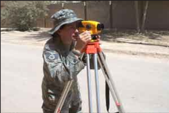
Photo by Lt. Col. Rhonda McGuire, JASG Public Affairs Staff Sgt. Tara Winder, an engineer with the JASG-C's Department of Public Works, uses an auto level to determine the amount of slope in a road near the New Embassy Complex.
