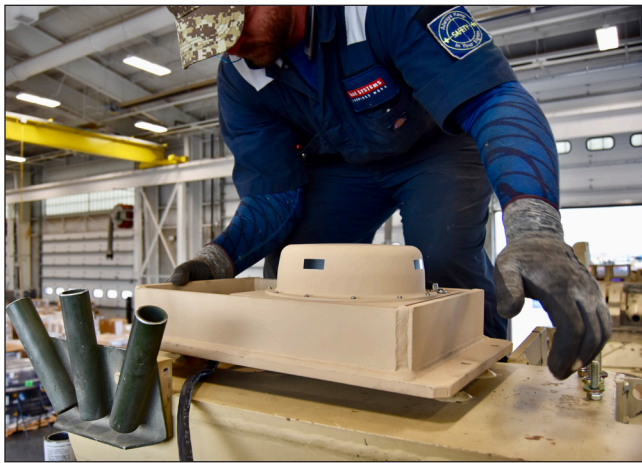
Timothy Stevens, a Heavy Mechanic from BAE Systems installs a Joint Battle Command-Platform transceiver on a M2A3 Bradley, July 17. The JBC-P is the Army's newest evolution of the Force XXI Battle Command Brigade-and-Below/Blue Force Tracking systems.
