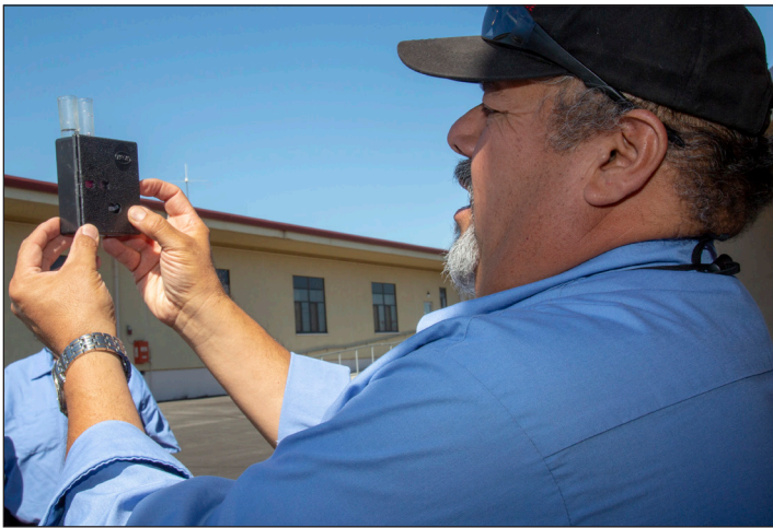
Paul Borrueal, utilities systems operator, dials in the device used to test water samples to ensure that they are at the correct level of detectable chlorine for Marine Corps Logistics Base Barstow, California, July 10.
