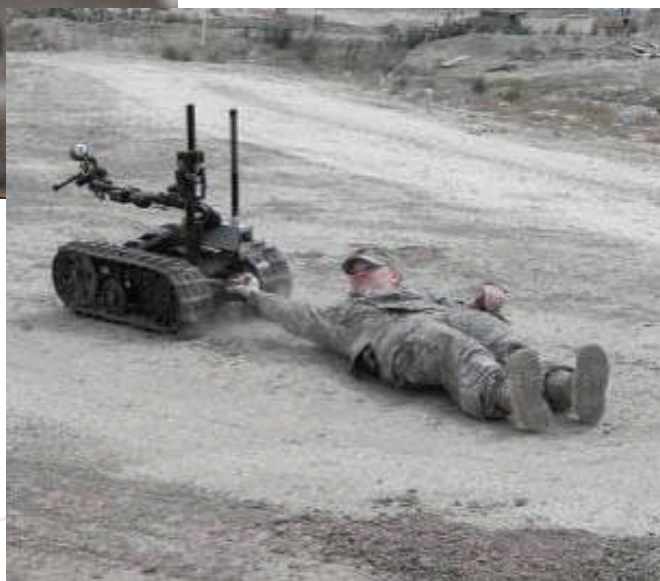
While being dragged, 225th Engineer Brigade Soldier Sgt. Kasandra Deutsch of Pineville, La., demonstrates the power of the Talon robot April 15 during a training exercise with the 9th Iraqi Army Engineer Regiment. The Talon robot system is used to help clear improvised explosive devices (Photo by Maj. Pat Simon).
