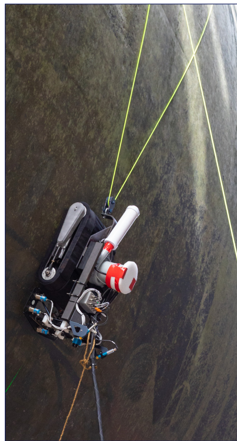
A hull-crawling robot scales the underside of USS Connecticut (SSN 22) to perform a hull inspection. (PSNS & IMF photo by Jeb Fach)
