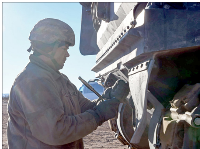
Spc. Geoff Adler, wheeled vehicle mechanic for Forward Support Company, 1-147th Field Artillery Battalion, South Dakota Army National Guard, utilizes a socket wrench to tilt the cab into a M270A1 Multiple Launch Rocket System in order to access the engine prior to the unit's validation training exercises.
