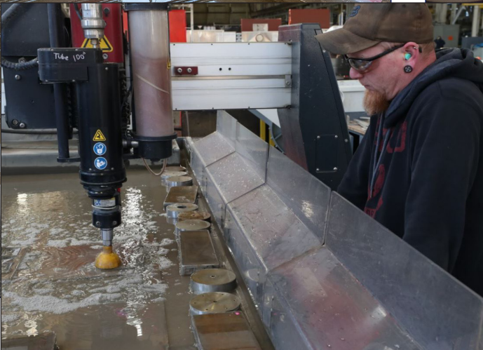
Michael Smith, Shop 11 shipfitter, watches the water jet cutter cut out a wrench from tool steel.
