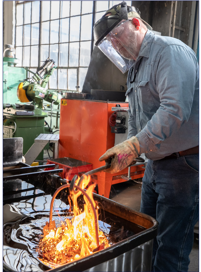
Erlend Frederickson, a Shop 11F heat treater, uses an oil bath to heat treat a batch of wrenches cut out on the water jet cutter. An oil bath is used to slowly cool the object versus water to avoid the wrenches from becoming too brittle to be used.
