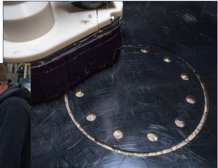
A computer-controlled router completes the final cut on a temporary hatch cover within 30 minutes of the steel original object being scanned.
