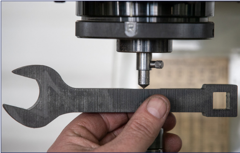
After a wrench is hardened in an oil bath and cleaned up, it is tested for hardness.
