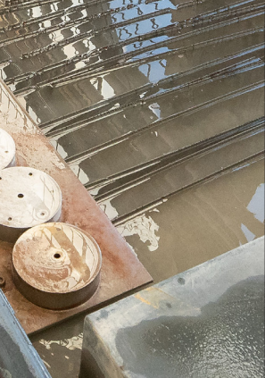
The computer-controlled water jet cutter uses a high pressure jet of water to cut through up to several inches of steel.
