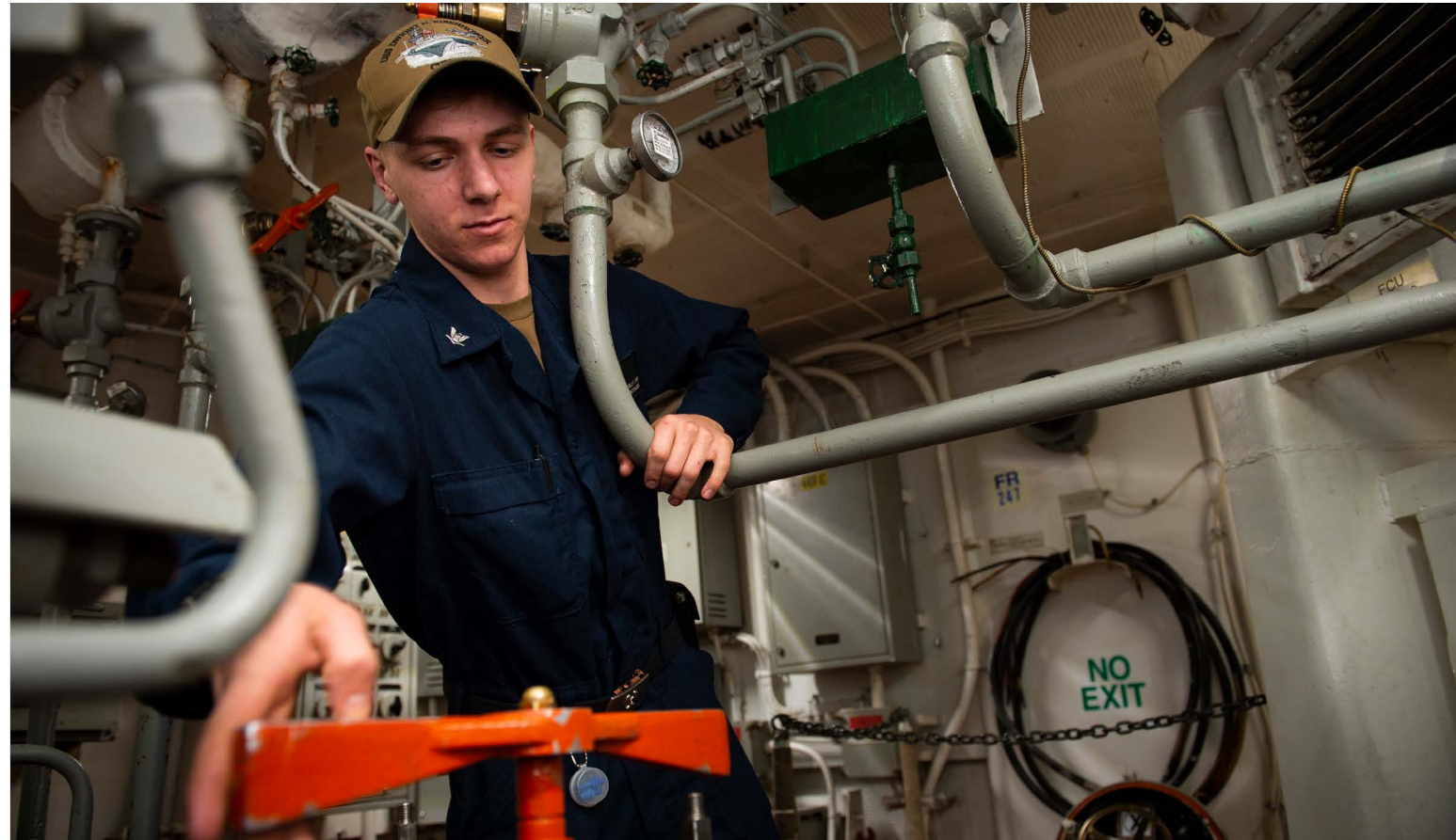
Machinist's Mate 3rd Class Niklas Ohiko aligns a fluid path of a steering gear unit in a steering gear room. Photo by MC3 Kaleb Sarten.
