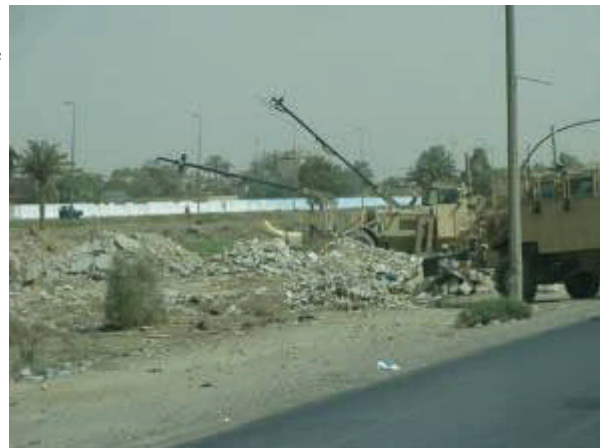
BAGHDAD – Soldiers of the 836th Engineer Company, from Kingsville, Texas, use the Husky and Buffalo to interrogate a possible improvised explosive device on Feb. 11. The 836th Eng. Co. is attached to the 890th Engineer Battalion, 225th Engineer Brigade, 1st Cavalry Division, Multi-National Division – Baghdad.
